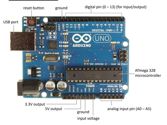
Arduino board connects input/output devices with two types of pin: digital pin and agalog input pin.
